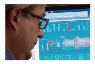
TIGER® continuously evaluates the state of gas and steam turbines by automating the knowledge of the best turbine engineers. By diagnosing the state of the turbine every second, a complete picture is built-up of the condition of the turbine. TIGER® performs several thousand fault detection steps every second.
